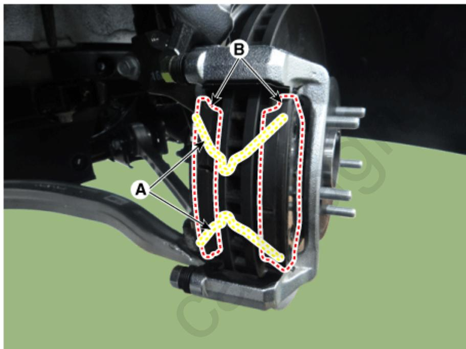
4. Loosen the brake member assembly bolts and then remove the brake member assembly.
