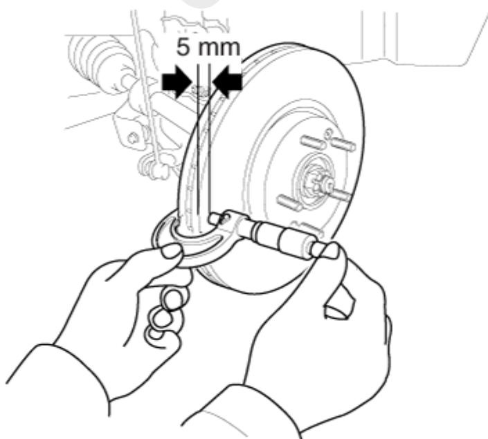
4. If wear exceeds the limit, replace the discs and pad assembly left and right of the vehicle.
