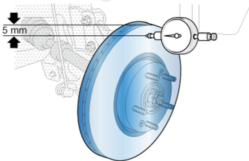
2. If the runout of the brake disc exceeds the limit specification, replace the disc, and then measure the runout again.
