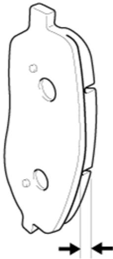
2. Check that grease is applied to sliding contact points and check the pad and backing metal for damage.
